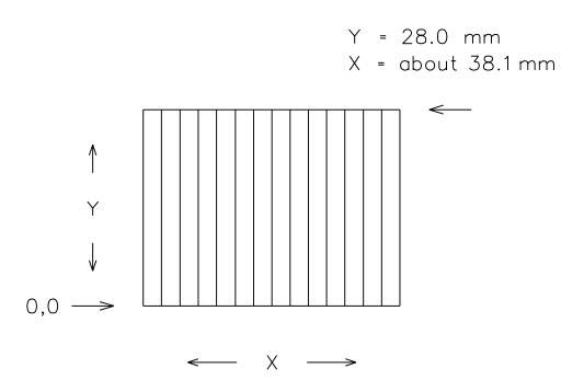
The extruded bar stock for these heat sinks is about 1.5" wide and comes in a 6 foot lengths.
