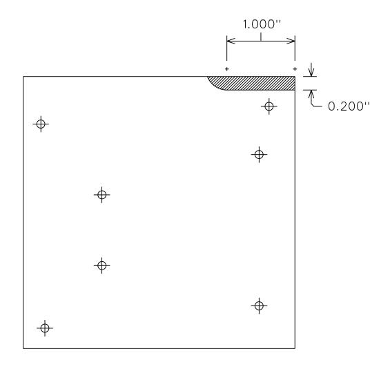
This drawing is looking at the flat thermal contact side of the Base Function Heat Sink.
