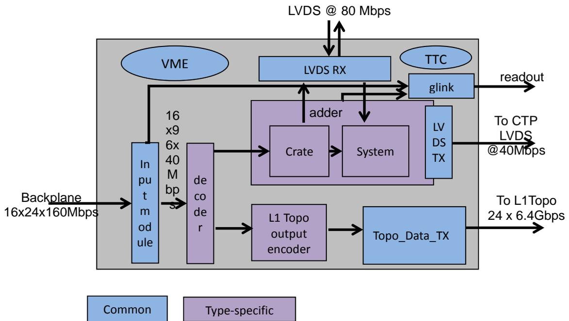
Figure 1: Conceptual diagram of the firmware modules and data flow between them
