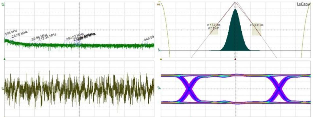
Figure 4. The scope tests of the optical output (an eye diagram) is presented. The rise and fall time is below 240ps.
