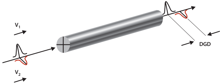
PMD (or differential group delay) effects on a fiber
