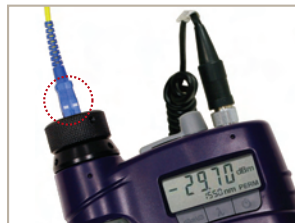
Patch cord inspection
