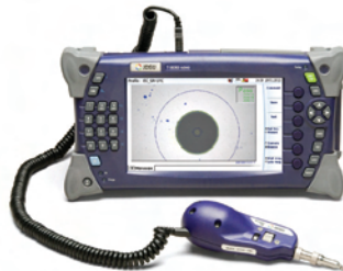
Pass/Fail image analysis on OTDR
