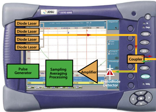
Figure 30: JDSU Pulse Delay OTDR method in the T-BERD/MTS-6000 platform
