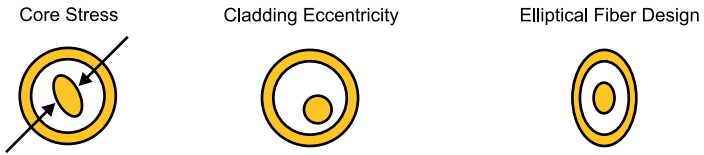
Figure 34: Imperfect fiber design causes birefringence
