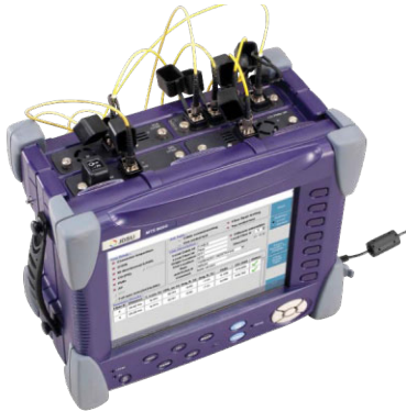
Figure 92: T-BERD/MTS-8000 configured with the MTAU module connected to the fiber characterization test modules
