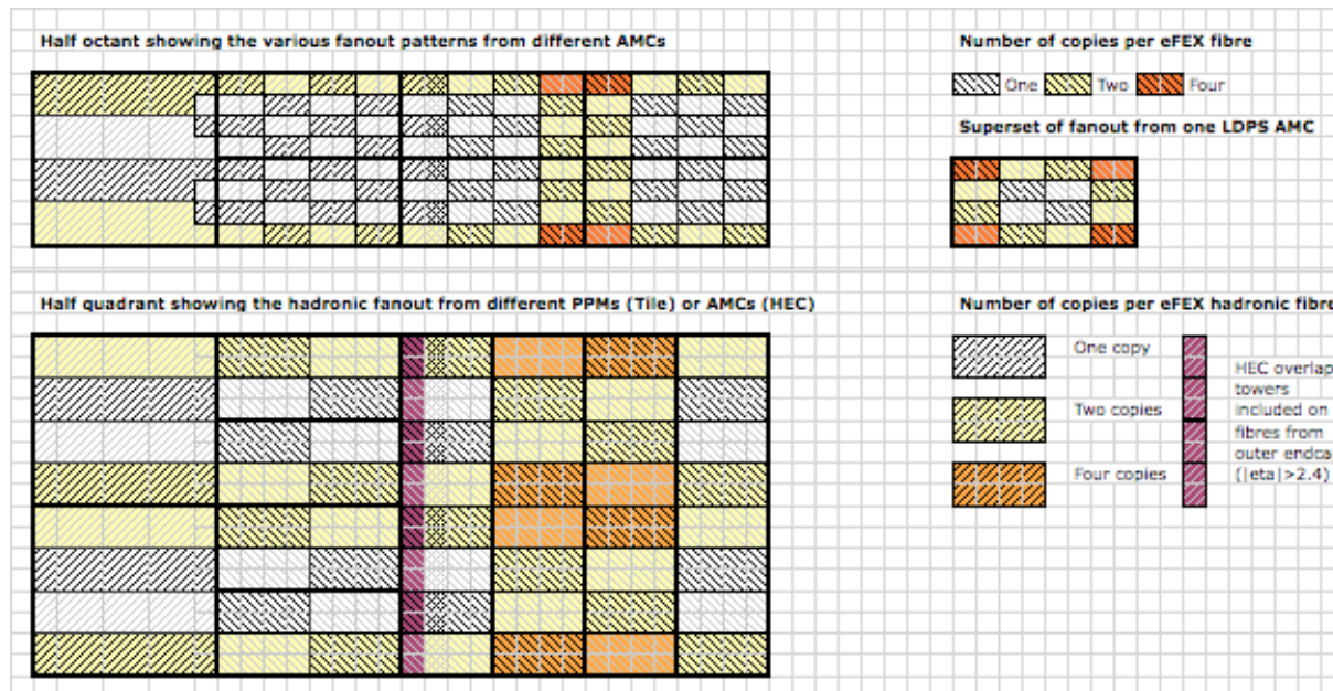
Figure 5: AMC fiber coverage and eFEX fanout requirements at 6.4 Gbit/s.
