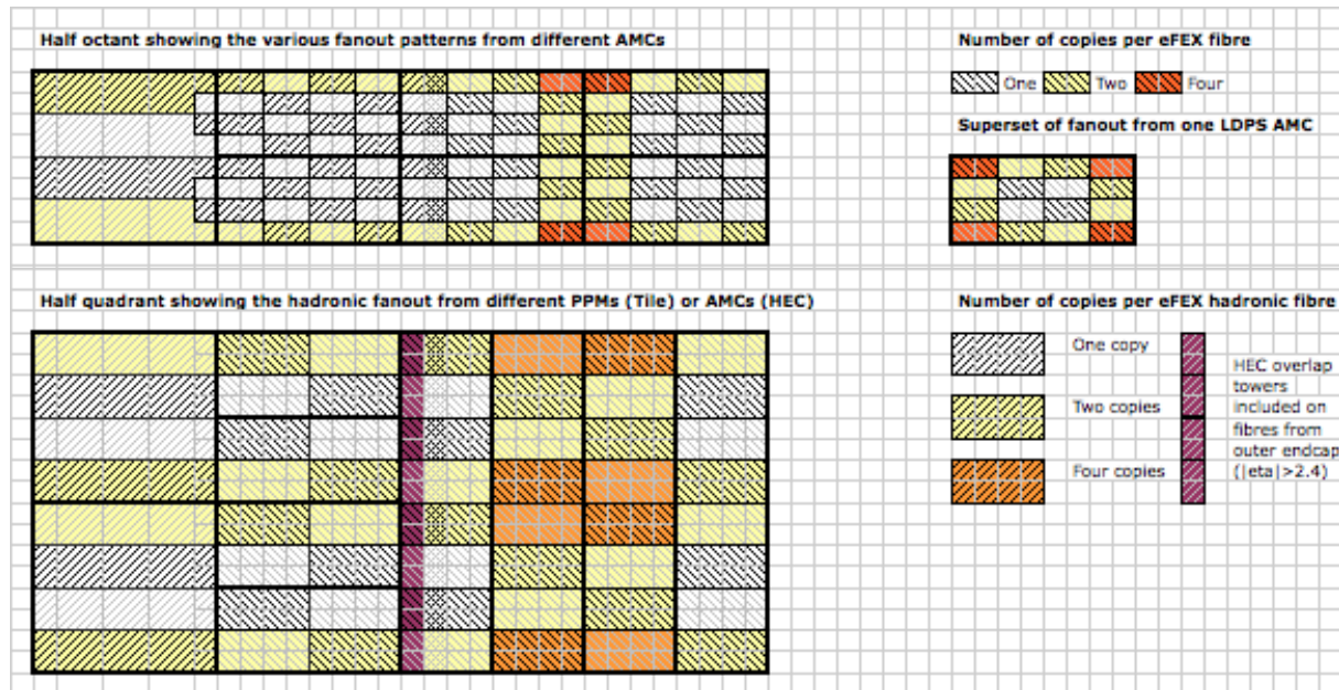
324 Figure 5: AMC fibre coverage and eFEX fanout requirements at 6.4 Gbit/s. Each square box corresponds to one trigger tower covering 0.1 \times 0.1 in \eta \times \phi . Each rectangular box corresponds to one fiber.
