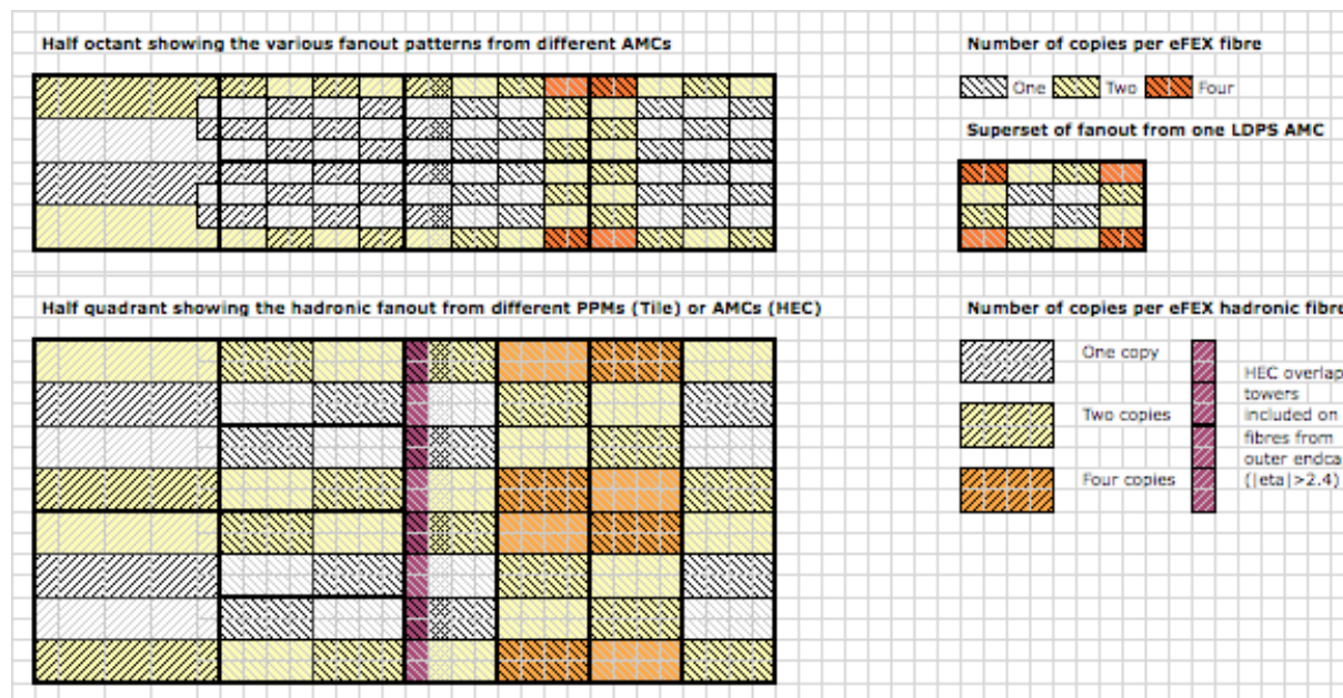
313 Figure 5: AMC fiber coverage and eFEX fanout requirements at 6.4 Gbit/s.
