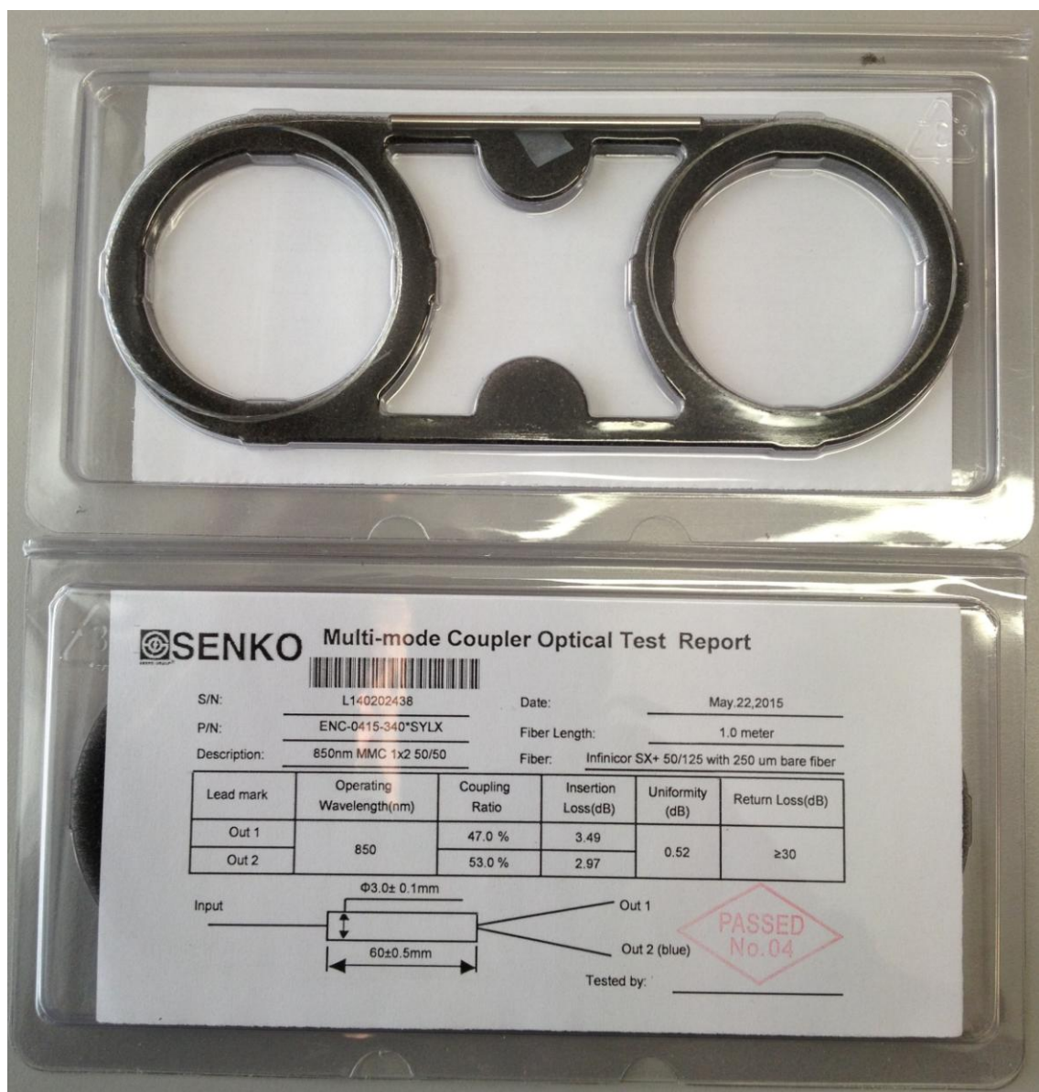
Figure 15: Passive splitter with bare fibers.
