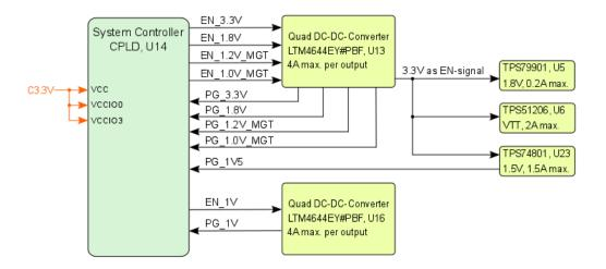
① To avoid any damage to the SoM, check on-board voltages in steady state before applying VCCIO voltages to the SoC's I/O banks.
