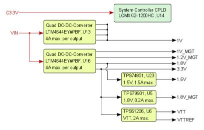
Power-on sequence is handled by the System Controller CPLD using "Power good"-signals from the voltage regulators:
