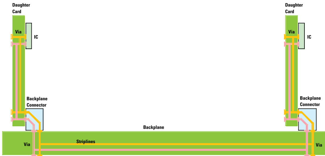
Figure 5-5. A Simplified Backplane Subsystem
