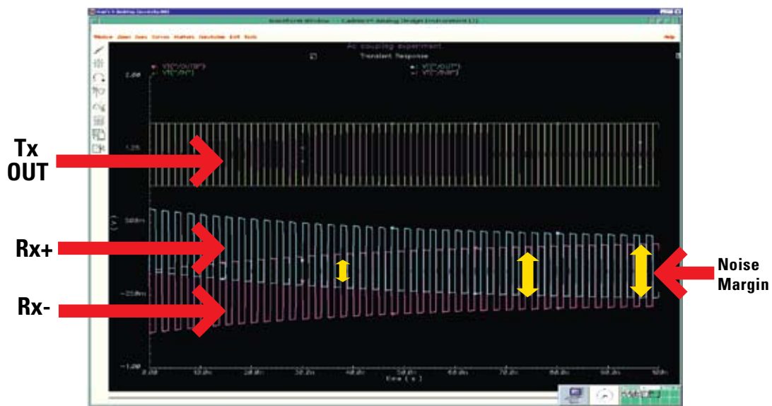
Figure 4-3. AC-Coupled Differential Pair at Startup
