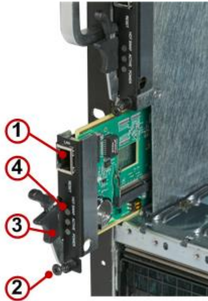
Figure 39: Shelf Manager Board Replacement
