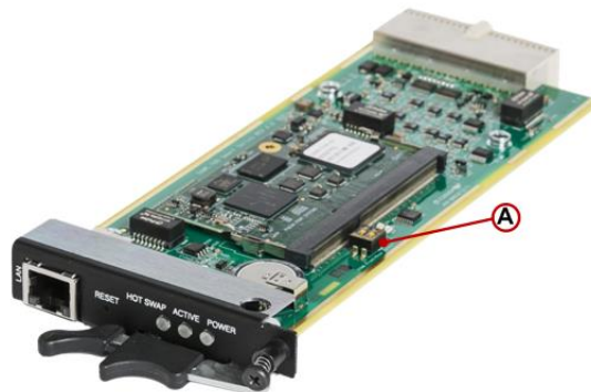
Figure 8: Dip Switch Location on the Shelf Manager Board
