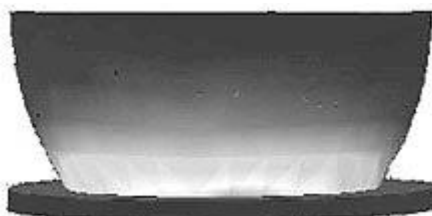
Figure 6. Example of the extensive FEA analysis to develop reliable joints between the solderball and PCB pad.
