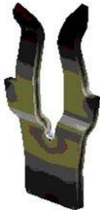
Figure 5. FEA model employed to develop the receptacle dual beam terminal.
