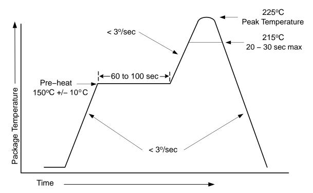
Figure 49. Soldering Temperature/Time Profile
