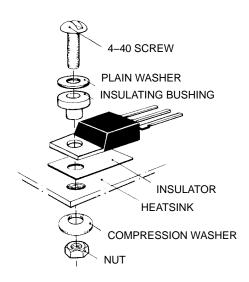
Figure 33. Screw-Mounted TO-220
