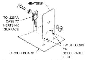
Figure 38. Simple Plate, Vertically Mounted
