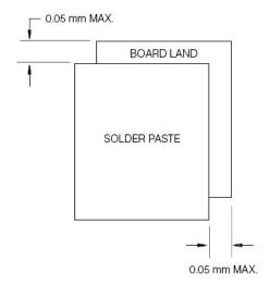
Figure 54. Solder Paste Application
