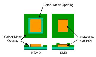
Figure 11. Comparison of NSMD vs. SMD Pads
