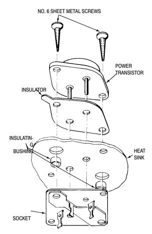
Figure 26. Hardware Used for a TO-204AA (TO-3)
