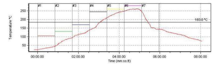
Figure 51. Lead-Free SAC 305 Solder Profile
