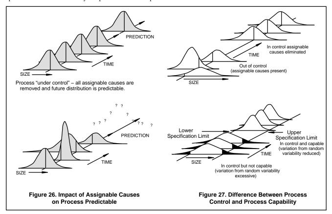
At ON Semiconductor, for critical parameters, the process capability is acceptable with a Cpk = 1.50 with continual improvement our goal. The desired process capability is a Cpk = 2 and the ideal is a Cpk = 5. Cpk, by definition, shows where the current production process fits with relationship to the specification limits. Off center distributions or excessive process variability will result in less than optimum conditions.
