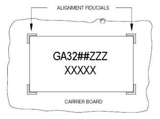
Figure 55. Alignment of Fiducials
