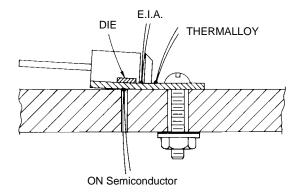
Figure 41. JEDEC TO-220 Package Mounted to Heatsink Showing Various Thermocouple Locations and Lifting Caused by Pressure at One End
