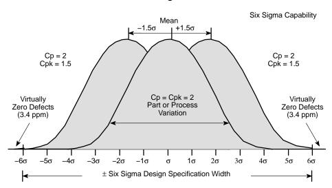
Figure 14. A Six Sigma Process Has Virtually Zero Defects Allowing for 1.5σ Shift
