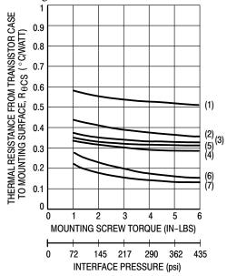
Figure 21. TO-204AA (TO-3) With Thermal Grease
