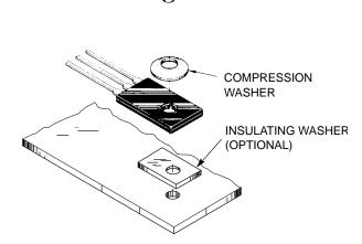
Figure 31. Eyelet Mounting
