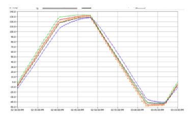
Figure 46. Typical Temperature Cycling Profile for Solder Joint Fatigue Testing
