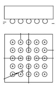
Figure 42. Daisy Chain Flip Chip CSP
