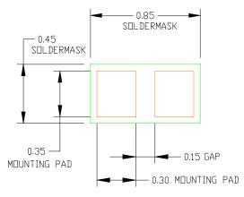
Figure 7. Maximum Recommended Mounting
