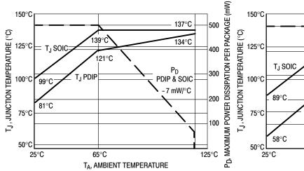
Figure 23. Junction Temperature for Worst Case CMOS Logic Device
