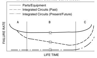
**Decreasing Failure Rate** Constant Failure Rate Increasing Failure Rate Infant Mortality Useful Life Manufacturing Variations Random (Chance) Defects Material, Design, Workmanship Defects (No Pattern: Occur Regularly) Weibull Weibull Weibull Log Normal Gamma Distribution Exponential for Equipment Log Normal for ICs Normal (Gaussian)
