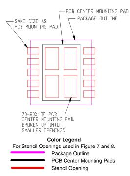
Figure 13. Typical for 0.5 mm Pitch or Greater DFN/QFN Package with Stencil Openings Shown Over PCB Mounting Pads
