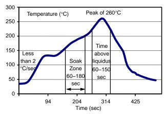
Figure 15. Typical Reflow Profile for Lead Free Solder
