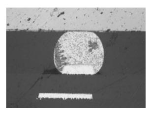
Figure 45. Cross Section of Flip Chip Solder Bump
