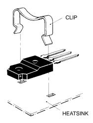
Figure 35. Clip-Mounted Isolated Package
