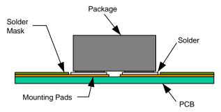
Figure 5. Cross-Section of Mounted Package
