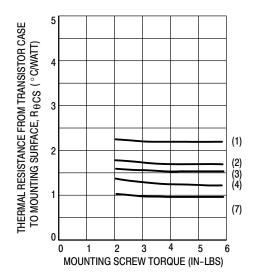
Figure 23. TO-220 With Thermal Grease
