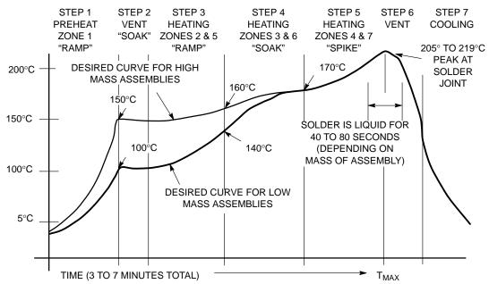
Figure 5. Typical Tin Lead (SnPb) Solder Heating Profile
