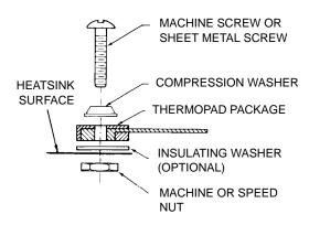
Figure 30. Machine Screw Mounting
