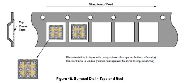
The SMD pick and place machines should pick up the component from the point which is located in the center of two adjacent sprocket holes in the feeding direction. This must be taken into account when designing the location of the component in the Tape and Reel pocket.
