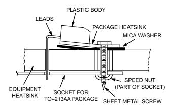
Figure 18. Extreme Case of Improperly Mounting a Semiconductor (Distortion Exaggerated)
