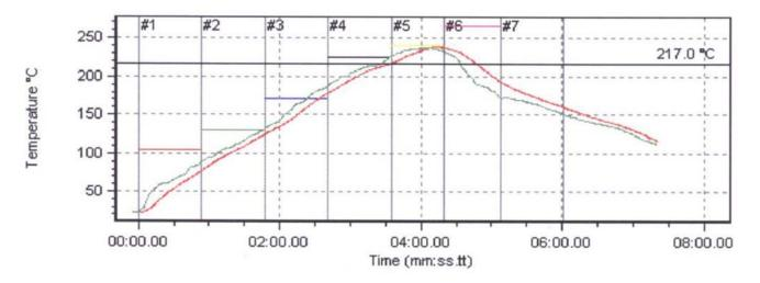
Figure 50. Tin/Lead Solder Profile
