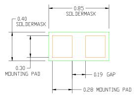
Figure 6. Recommended Mounting Pattern
