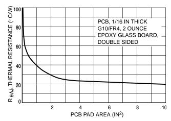
Figure 37. Effect of Footprint Area on Thermal Resistance of DPAK Mounted on a Glass–Epoxy Board
