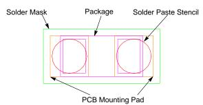
Figure 4. Recommended Mounting Pattern
