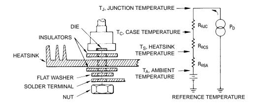
Figure 40. Basic Thermal Resistance Model Showing Thermal to Electrical Analogy for a Semiconductor
