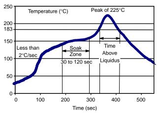
Figure 16. Typical Reflow Profile for Eutectic Tin /
