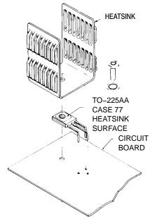
Figure 39. Commercial Sink, Horizontally Mounted
