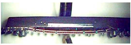
Figure 34. BGA Cross Section Exhibiting Moisture Damage (Popcorning)
