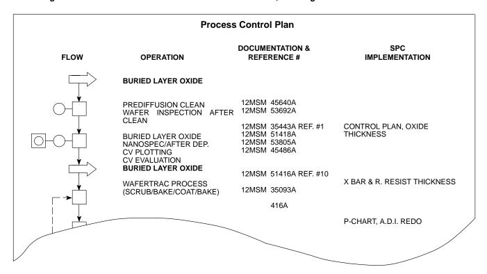
Figure 18. Part of a Wafer Fab Control Plan, Showing Statistical Process Control Details
