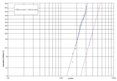
Figure 47. Weibull Plot of 400 μm/500 μm Pitch Daisy Chain Device Cumulative Temp Cycle Failure Rate
