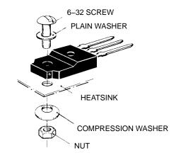
Figure 34. Screw-Mounted Isolated Package
