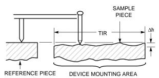
Figure 19. Surface Flatness Measurement
