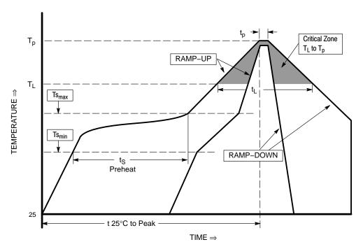
Figure 6. Typical Pb-Free Solder Heating Profile
