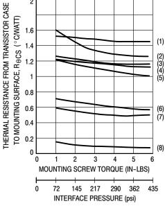
Figure 20. TO-204AA (TO-3) Without Thermal Grease
