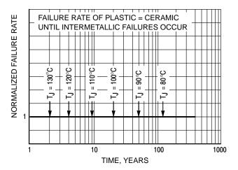
Figure 22. Failure Rate versus Time Junction Temperature
