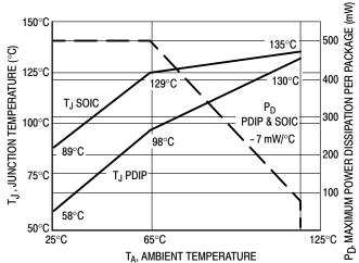
Figure 24. Junction Temperature for Typical CMOS Logic Device
