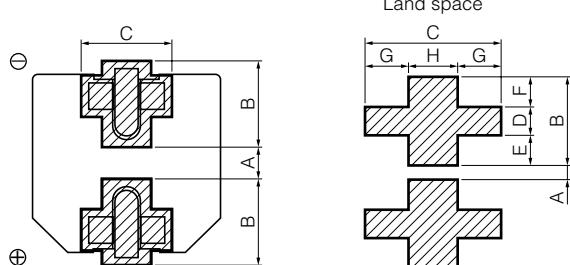
[Table of Board Land Size vs. Capacitor Size] (Unit : mm)
