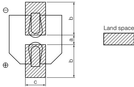
[Table of Board Land Size vs. Capacitor Size] (Unit : mm)
