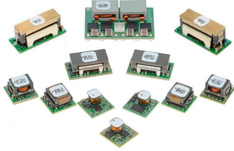
GE Energy POL power converters provide small, efficient, and reliable power electronics modules for FPGAs and DSPs. Our high-density POL (point-of-load) DC-DC converters provide a cost-effective solution to power silicon that includes DSP Core and I/O requirements ranging from 0.45 to 5.5V.
