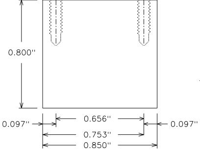
The two holes are drilled and tapped for 2-56 with 1/4" minimum of good threads.
