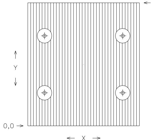
From the bar stock cut the heat sink blank Y dimension to a length of 110 mm.
