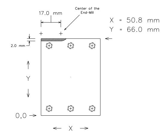
This drawing is looking at the flat thermal contact surface of the Fill Block with its six larger diameter hole recesses facing down.
