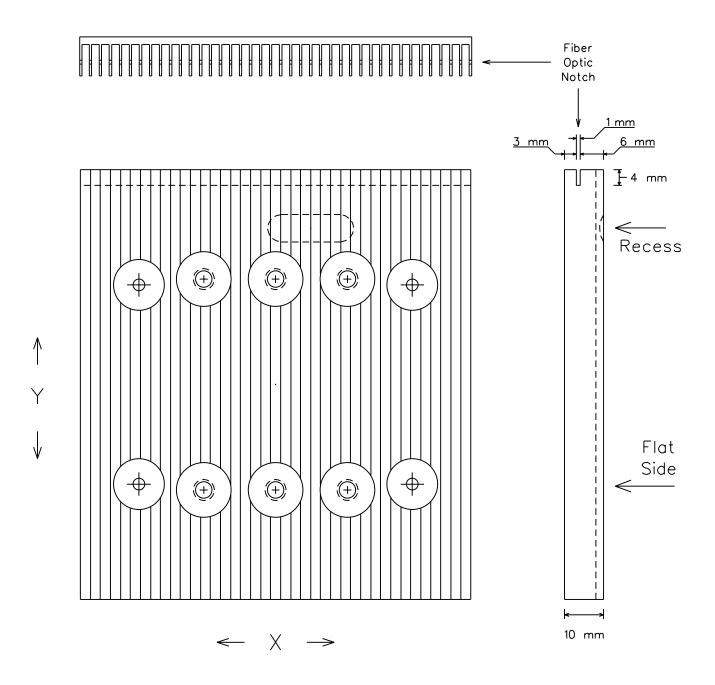
Please EDM a Fiber Optic Notch that is 1 mm wide and 4 mm deep through all 40 fins at the same end of the heat sink that has the ball mill recess in its flat side.
