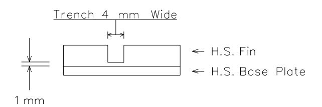
In a "trench" about 4.0 mm wide cut down the height of the fins so that they only reach about 1.0 mm above the base plate of the heat sink.
