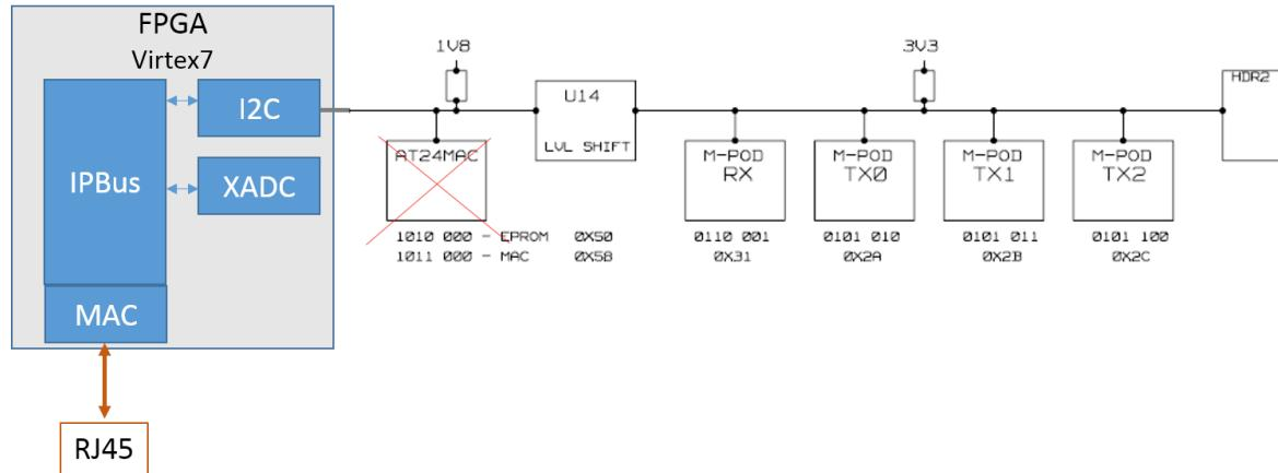
The ROD IPbus monitoring targets include the ROD FPGA XADC, one Rx and three Tx MiniPODs (temperature and voltage) sharing one I2C bus. The novo memory chip on the I2C bus can be ignored by DCS.
