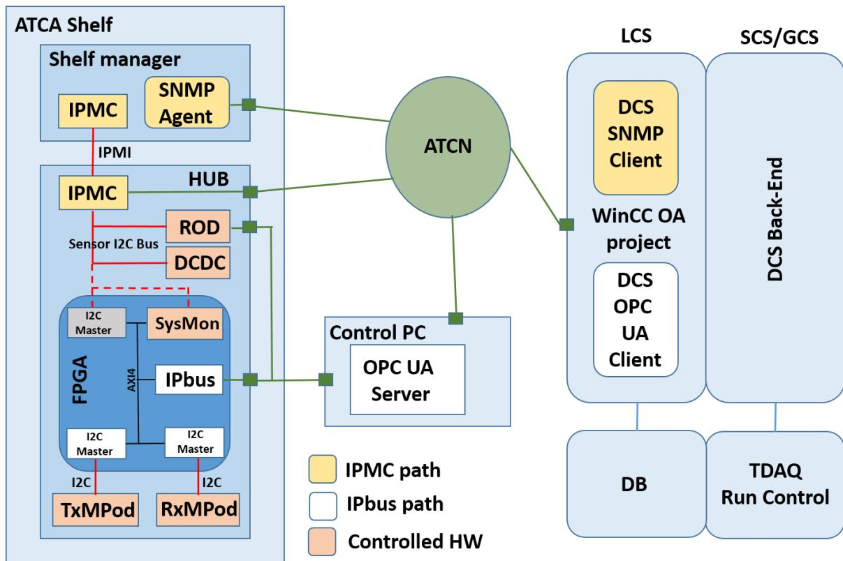
The controlled hardware components of the HUB/ROD module in the ATCA shelf are accessible for DCS control and monitoring via two paths:
