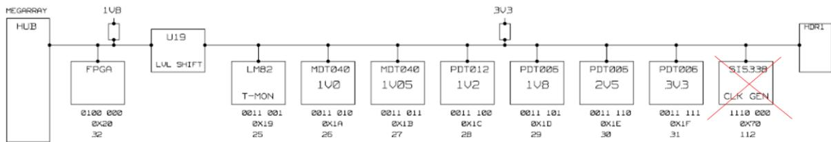
The IPMC card on the HUB via the Sensor I2C Bus (on the left side on the above diagram) can access an LM82 temperature sensor and six DCDC converters (temperature and voltage). The clock chip on the Sensor I2C bus can be ignored by DCS monitoring.
