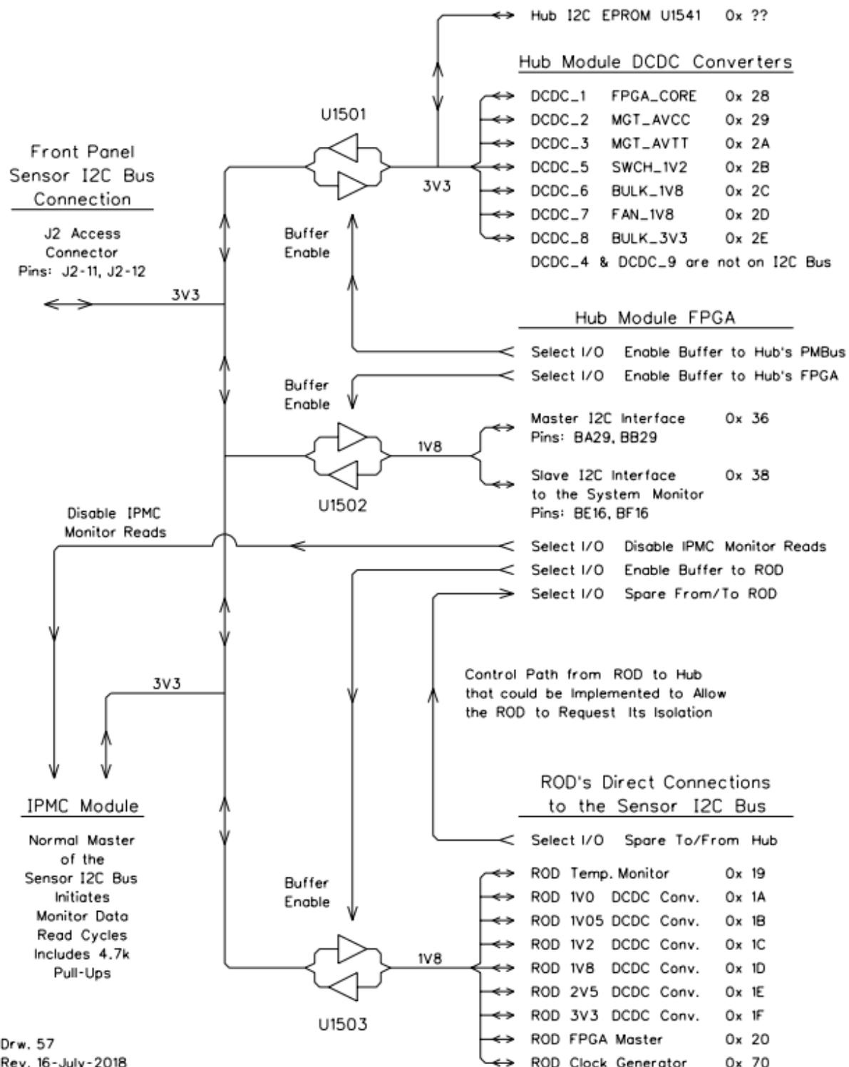
ROD Sensor I2C bus structure for IPMC Monitoring is shown below:
