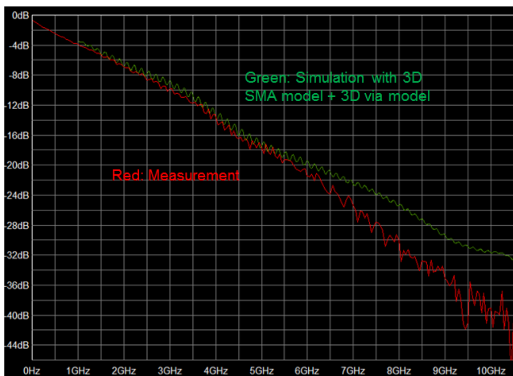
Figure 8. PCB S-parameter simulation and measurement
