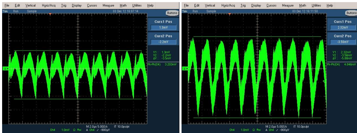
Figure 9. HSD Xilinx GTH power supply noise (Left, 3.2mV pk-pk on 1.0V MGTA VCC; right 4.8mV pk-pk on 1.8V MGTA VCC PLL)
