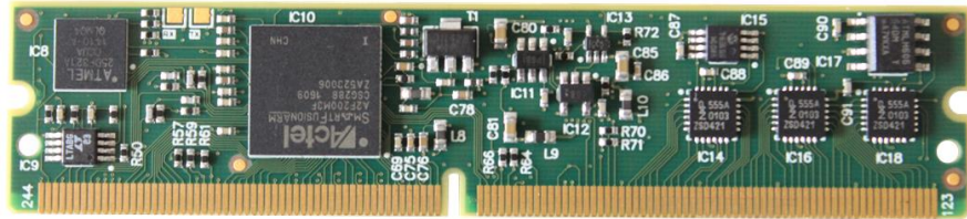
Second revision of the CERN IPMC mezzanine
