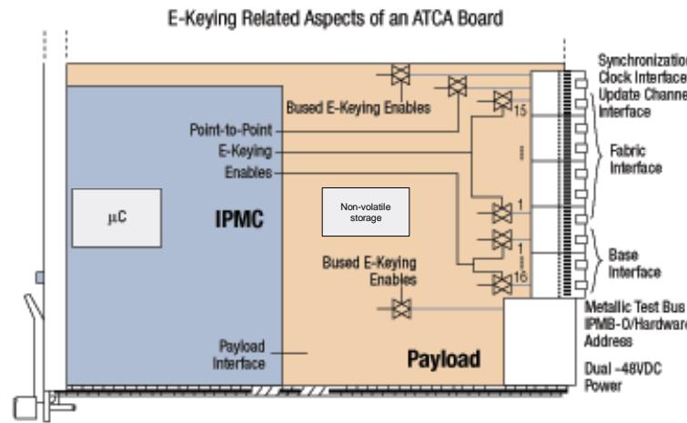
The board's non-volatile storage include FRU information with E-Keying data (i.e. link descriptor). The Shelf Manager use these information to managed the P2P connections to the backplane.
