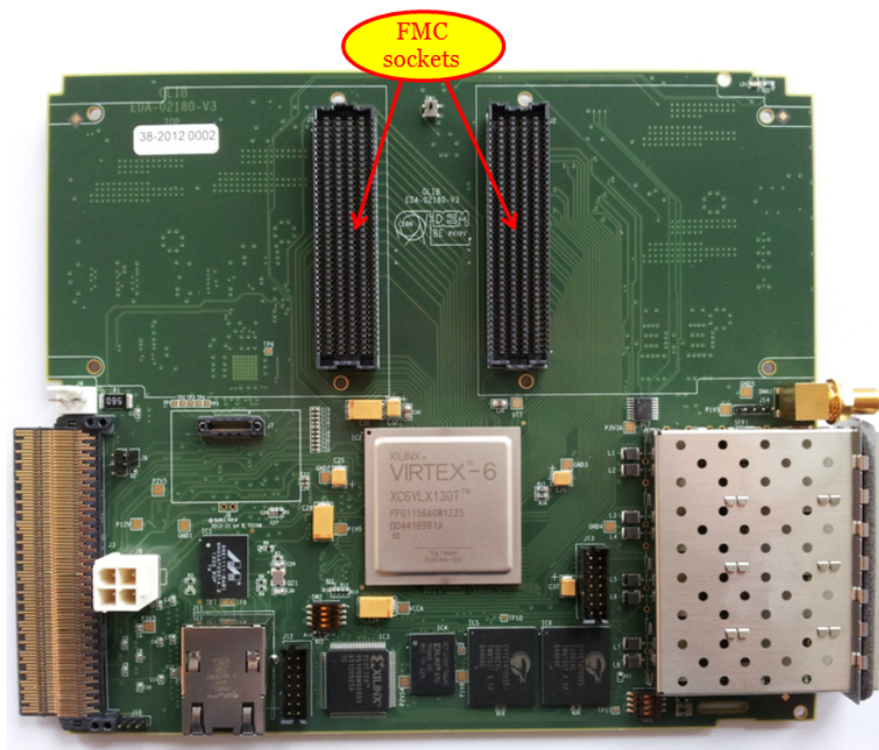
Figure 2. Picture of the GLIB AMC, highlighting the two FMC sockets.
