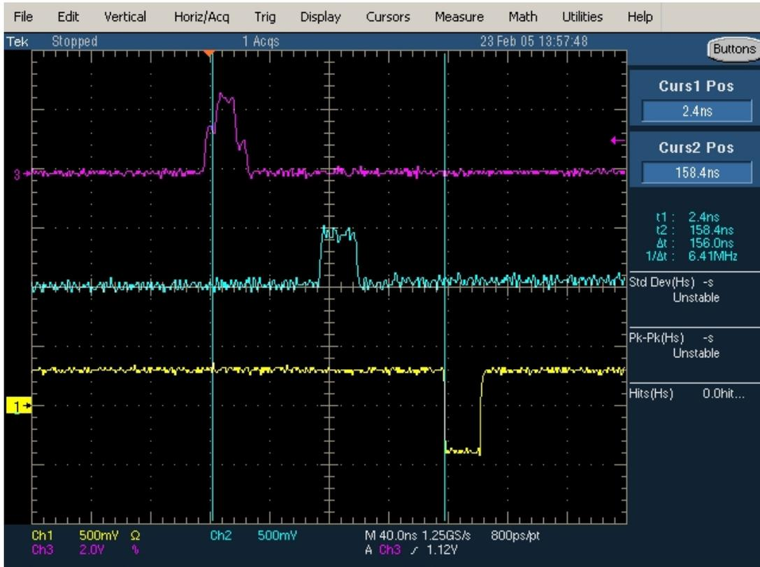
Figure 9: CMM latency. The upper trace is the CPM hit output, measured at the rear of the CPM. The middle trace is the CMM crate-summing output, measured at the rear of the CMM RTM. The bottom trace is the system-summing CMM output to the CTP. Traces 1 and 2 used single-ended probes, trace 3 used a differential probe.
