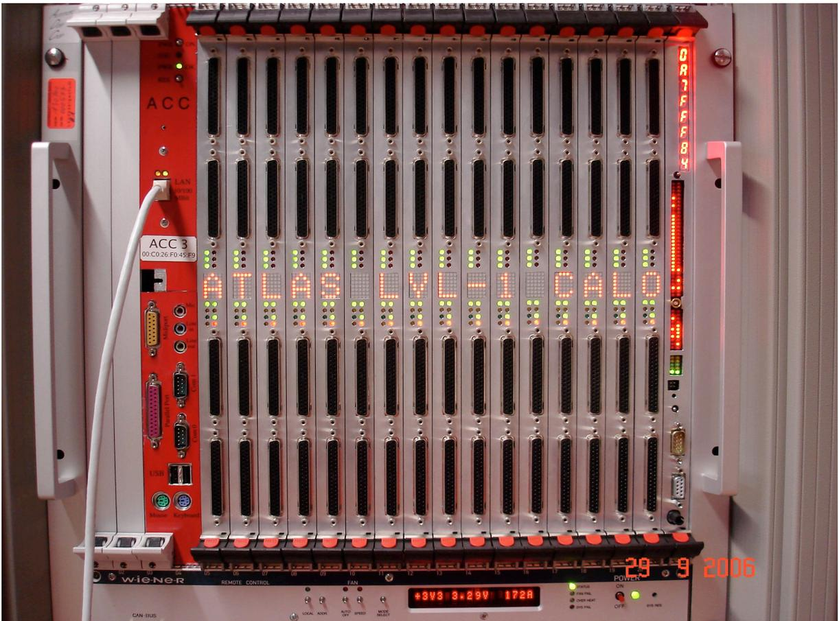
Figure 21 : The fully-assembled PPr-crate with a TCM, 16 PPMs and a 9u VME-CPU.
