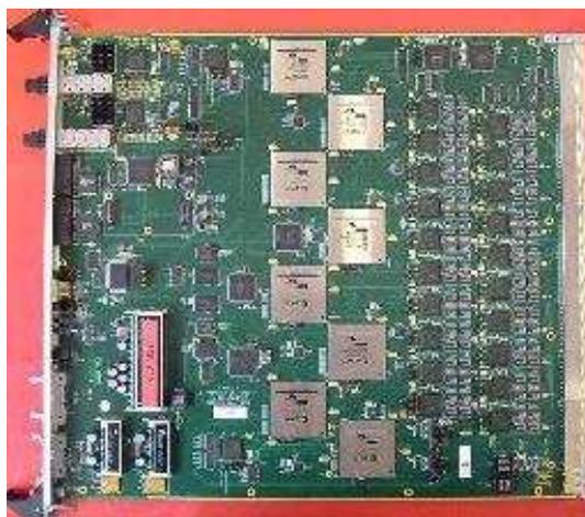
**Figure 18.** Photograph of a CPM. From right to left, de-serialiser and serialiser chips, 8 CP chips, optical readout to DAQ and L2.
