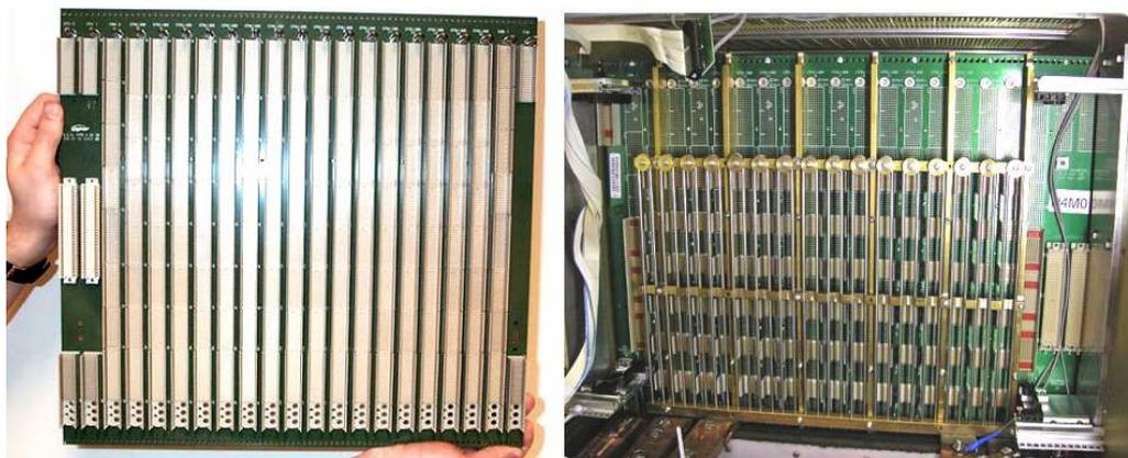
**Figure 25.** Photographs of the Processor Backplane. Left: module side, with CPU connections in slots 1 and 2 and TCM in slot 21. Right: from rear of crate, showing cable supports for LVDS serial links into CPMs and JEMs.
