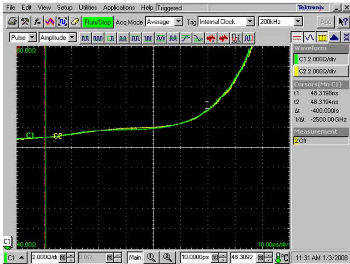
Figure 13. Skew Between Zig-Zag Traces
