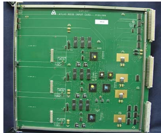
Figure 3: RoIB Input Card
