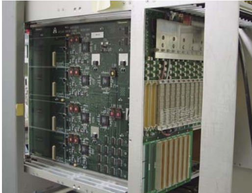
Figure 7: View of the fully populated RoIB crate
