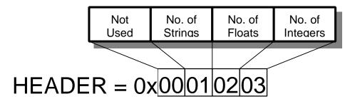
This header is compared against the actual number of each data type which are found and if there is a difference and error is generated.
