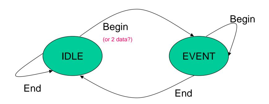
State bit (IDLE/EVENT) is input to FIFO handling logic
