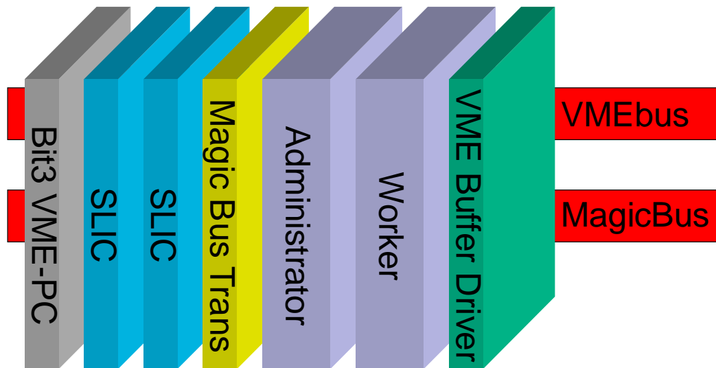
Figure 1: Picture showing the composition of a level 2 crate. The processors are contained in the SLIC, Administrator and Worker cards.
