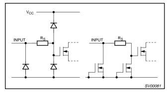
Figure 2. ESD Protection Circuits
