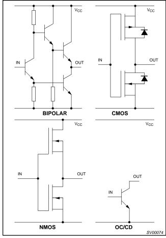
Figure 4. Typical digital output structures
