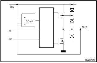
Figure 8. LVT's Output Circuit
