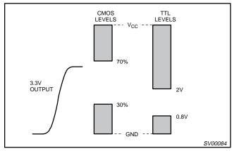
Figure 1. Switching Levels
