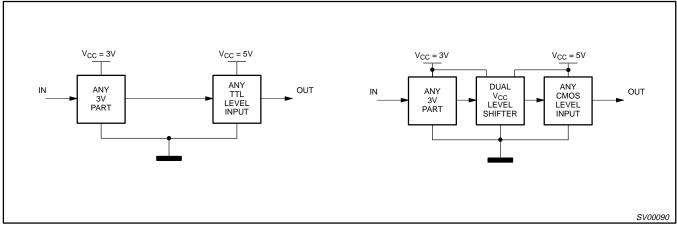
Figure 12. 3V Drivers to 5V Receivers
