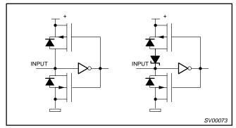
Figure 3. Bus hold circuits
