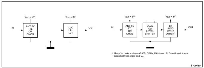
Figure 11. 5V Drivers to 3V Receivers
