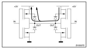
Figure 5. Currents from +5 to +3V
