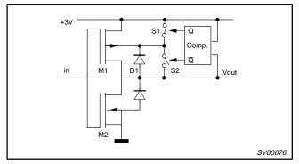
Figure 7. New LVC Output Structure
