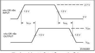
Waveform 1. Input to Output Propagation Delays
