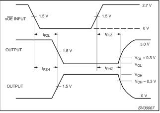
Waveform 2. 3-State Output Enable and Disable Times
