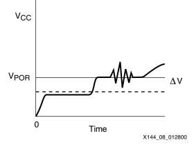
Figure 8: Noise on Top of V<sub>CC</sub>
