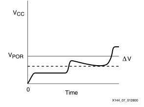
Figure 7: Non-monotonic V<sub>CC</sub>
