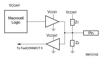
Figure 1: Simplified XC9500XL I/O Structure
