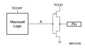
Figure 4: Close-Up View of Simplified Output Stage (ESD Circuits Not Shown)
