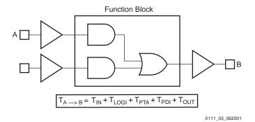
Figure 3: T<sub>PD</sub> with Initial Cascaded P-Terms
