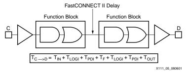
Figure 5: T<sub>PD</sub> with Multiple Pass Logic
