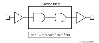
Figure 2: Simple T<sub>PD</sub> Example
