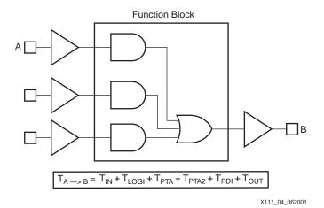
Figure 4: T<sub>PD</sub> with Initial Cascaded P-Term from Two Levels
