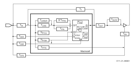
Figure 1: XC9500XL Detailed Timing Model
