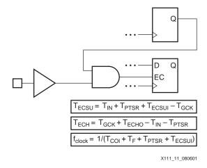
**Note:** Product term allocator delays ( $T_{PTA}$ ) and low power logic delays ( $T_{LOGILP}$ ) do not apply to Clock Enable timing calculations.
