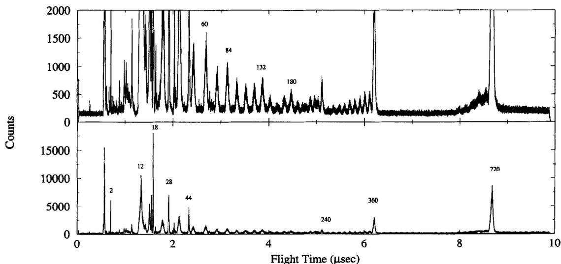
Fig. 2. Time-of-flight spectrum for positive fragments arising from bombardment of  $C_{60}$  by 625 MeV  $^{136}\text{Xe}^{35+}$  ions. The numbers given above some of the peaks are the ratios ( $M/Q$ ) of fragment mass (amu) to charge.
