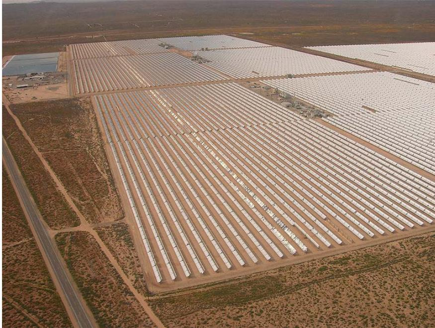
**Figure 4-10. Aerial View: Solar Thermal Power Trough Mirror Plant**
