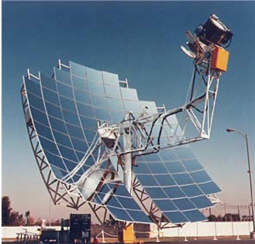
**Figure 4-12. Solar Sterling Engine on a Parabolic Reflector Dish**
