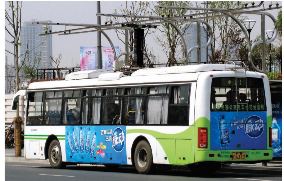
FIGURE 24.33 Supercapacitor-powered bus recharging at a bus stop in Shanghai, China.
