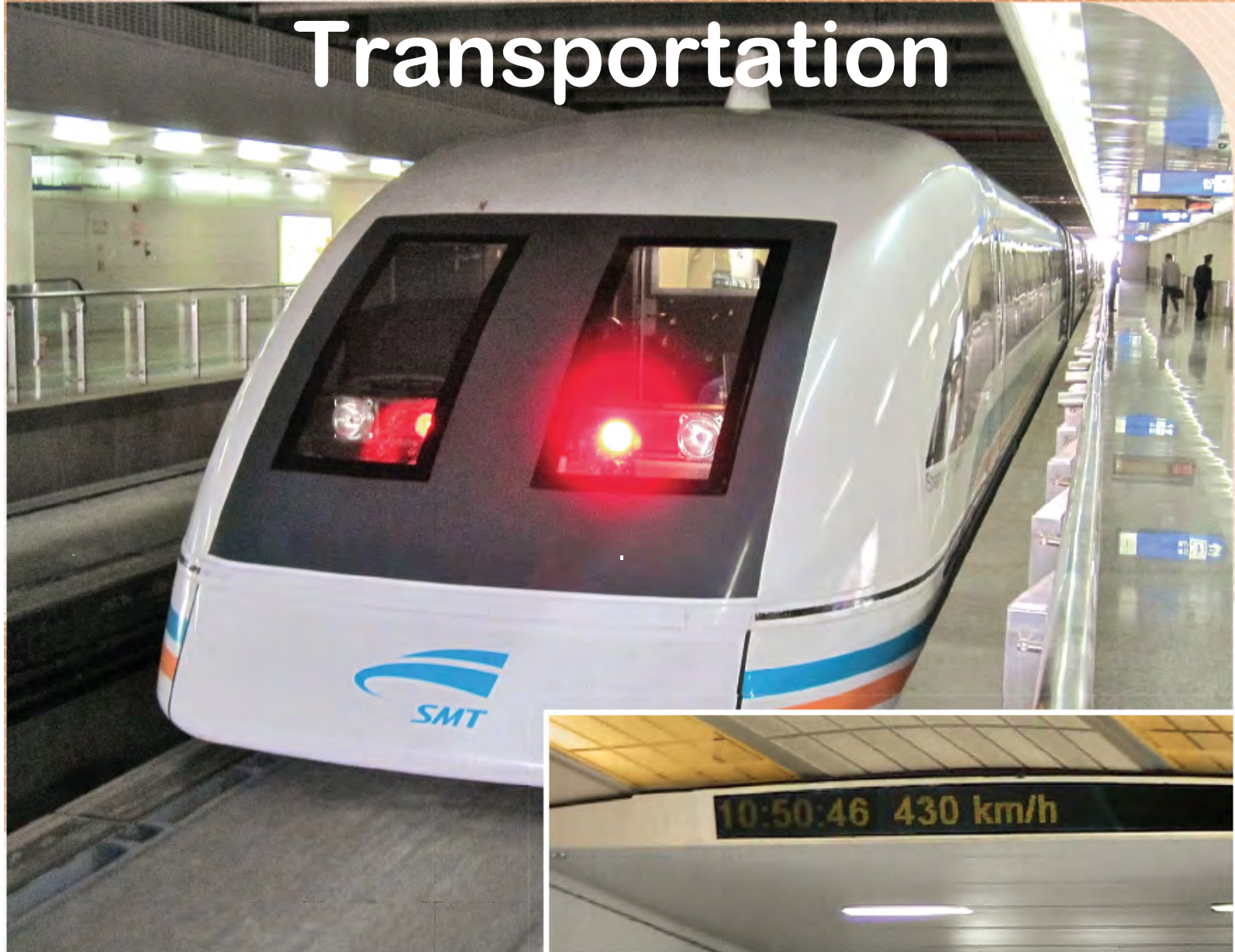
FIGURE 27.1 The Shanghai Maglev Train in the Pudong Airport station. The inset is a display inside the train showing the maximum speed of 430 km/h (267 mph) attained during the 7-minute 20-second trip from the airport to downtown Shanghai.
