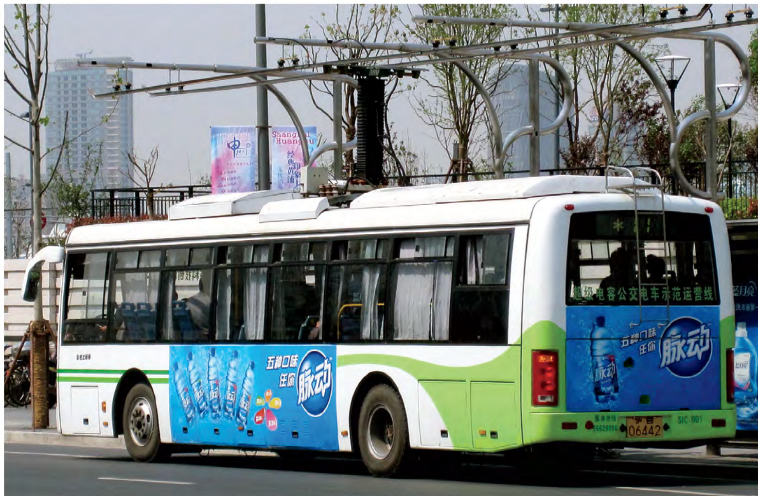
FIGURE 24.33 Supercapacitor-powered bus recharging at a bus stop in Shanghai, China.
