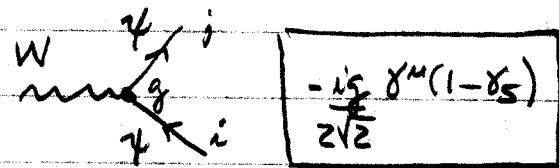
$$\mathcal{L} = -i \frac{g}{2\sqrt{2}} : \bar{\psi}_j \gamma^\mu (1-\gamma_5) \psi_i W_\mu : \quad i+j$$
