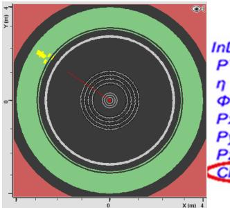
InDetTrack index: 2 PT=42.530 GeV η = 0.753 Φ = 145.560° Px=-35.075 GeV Py=24.052 GeV Pz=35.162 GeV Charge = -1 Track in the tracking detector
