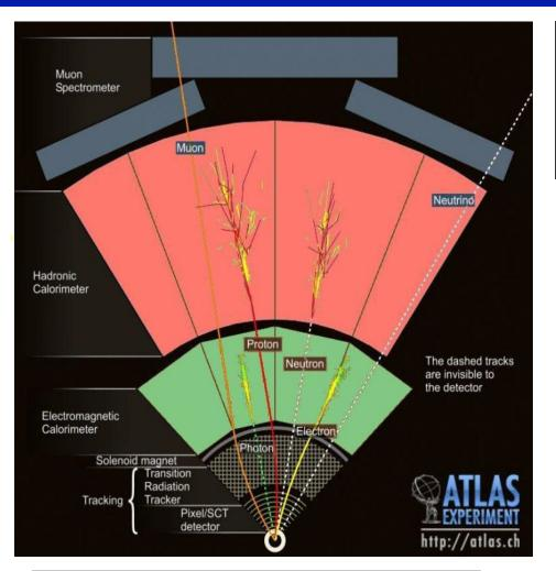
Neutrinos are only detected indirectly via 'missing energy' not recorded in the calorimeters
