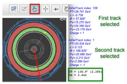
Hold the P key on the keyboard down and click on the two tracks (both turn into grey). The angle between both tracks in transverse plane is displayed in the Output box (green frame).
