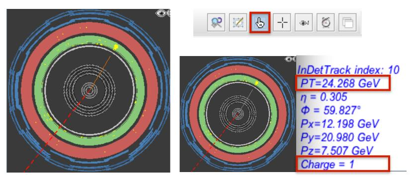
Here is the problem: determine the electric charge and momentum of the electron-like particle in this event display. Click the Pick symbol from the tool box, select the track (colour turns into grey) and look at the output box ...
