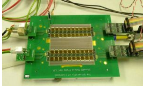
Figure 5. ATLAS Upgrade sensor module on a test board. A stave will have 24 such modules per side.
