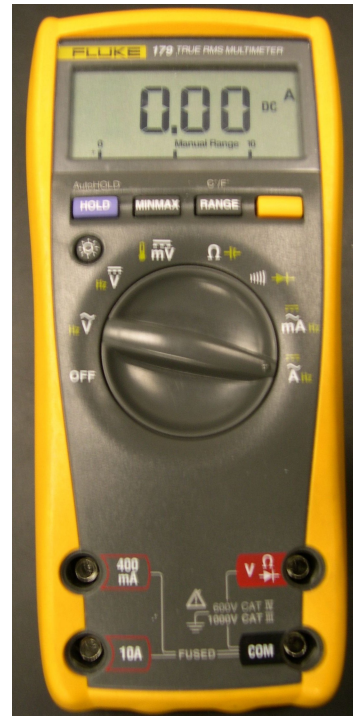
Figure 1.2: Digital multi-meter
