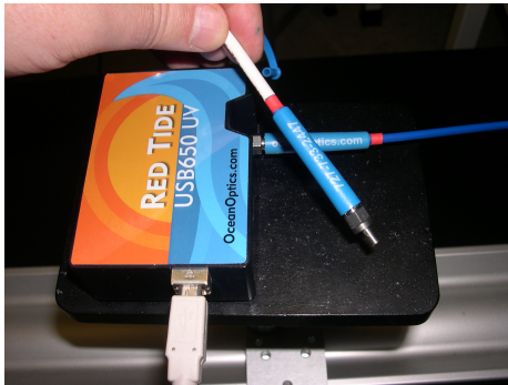
Figure 9.1: Digital spectrometer. Note the white USB cable and blue optical fiber.
