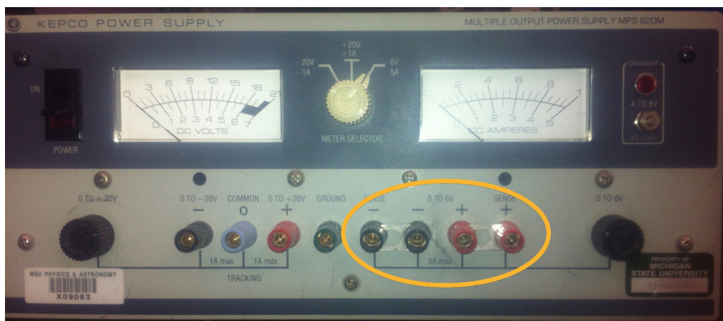
Figure 3.3: The power supply is a high-current device. We'll use the 6V, 5A maximum scales which reads on the bottom of each of the windows. You connect to the resistor through the sockets on the top of the calorimeter and to the + and - "0 TO 6 V" connectors on the front (circled).
