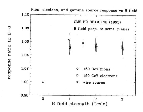
Fig. 4. Effect of a B field on the average energy response of the tile/fiber calorimeter to pions, electrons for H2(1995) data, and a calibration source. Here the B field lines are perpendicular to the scintillator plates (endcap configuration). In this configuration, the only effect is scintillator brightening with B field, which is the same for muons. hadrons, electrons and gamma rays from a radioactive source.
