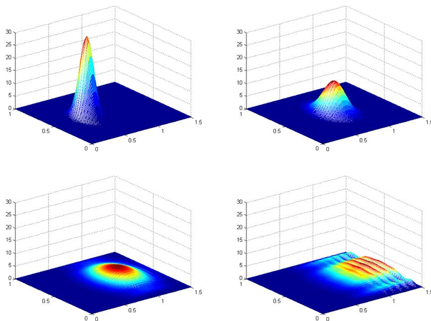
**Fig. 9:** Free propagation and reflexion of a 2D Gaussian wave packet. The figures from left to right show  $|\psi(x, y, t)|^2$  at time steps 1, 500, 1000 and 1300 when reflexion on boundary infinite walls occurs.
