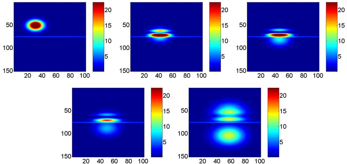
**Fig. 11:** Dynamics of 2d tunnel effect in non-peculiar incidence, investigated with 2d RK4 solver. Here is displayed  $|\psi(x, y, t)|^2$  at time steps 1, 300, 400, 500 and 700. On the last plot, the amplitude has been multiplied by 10 in order to be more visible.
