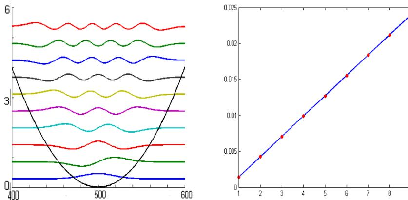
**Fig. 6:** Left: 10 first eigenvectors of the harmonic oscillator. The quadratic potential is represented in blue. The eigenvectors are shifted by their eigenvalues. Right: the red dots represent the 10 first numerically calculated eigenvalues and the blue curve is the expected analytical evolution  $E = \omega(n + 1/2)$  and  $n = 0, 1, 2 \dots$
