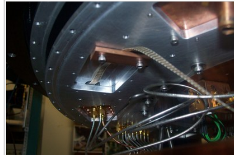
Channel for ribbon cable is milled in bottom of port cover
